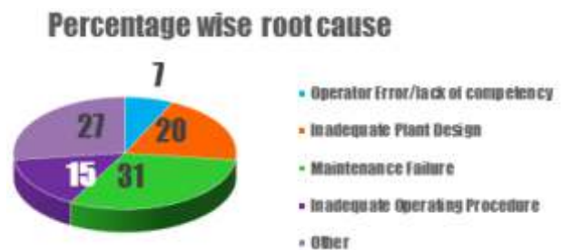
Figure 4 Causes of industrial fires
