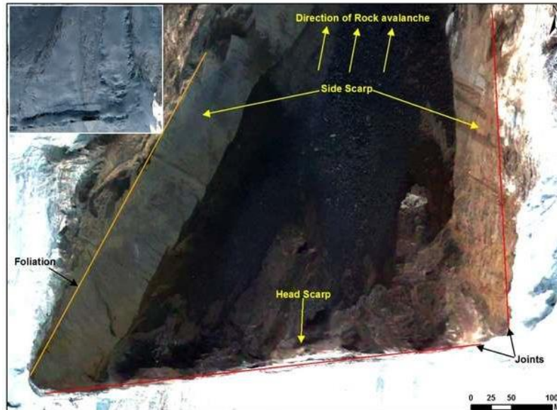
Figure 16: Post-failure Pleiades image showing the crown of the rock avalanche. Scarps exposed due to wedge-type failure along joint and foliation planes are seen. Inset shows pre-failure Komsat-3A image
