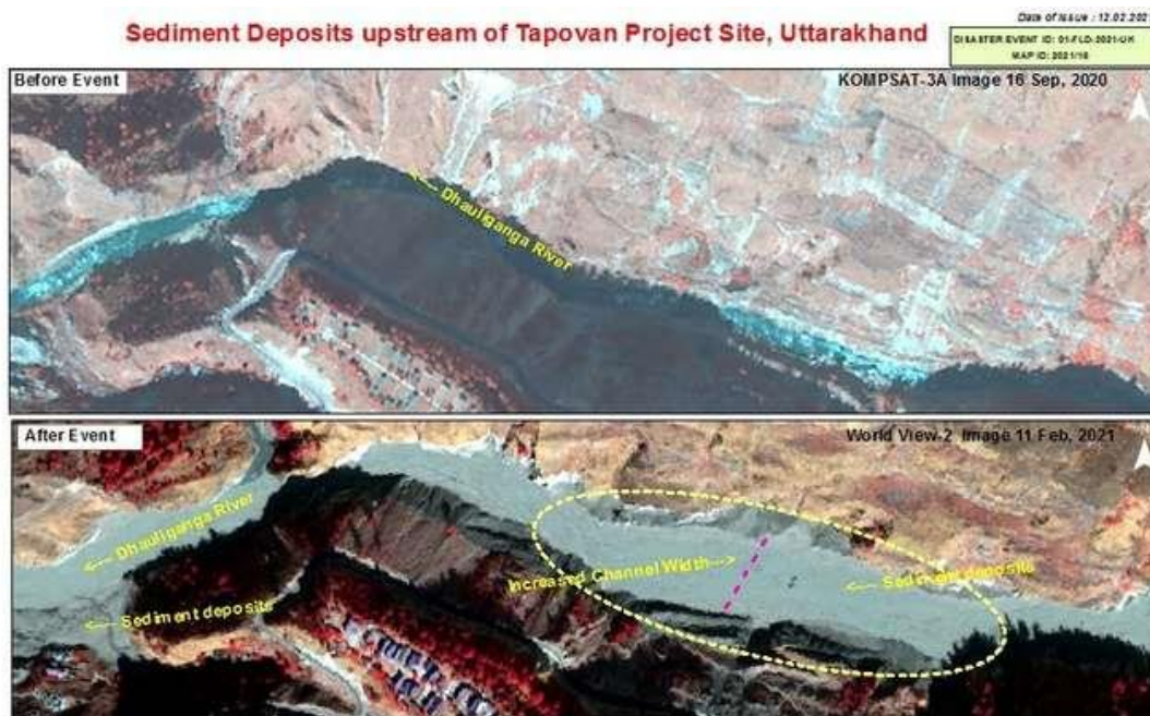
Figure 15: Damages to bridges and increased channel width in Tapovan Upstream (Source: NRSC-ISRO)
