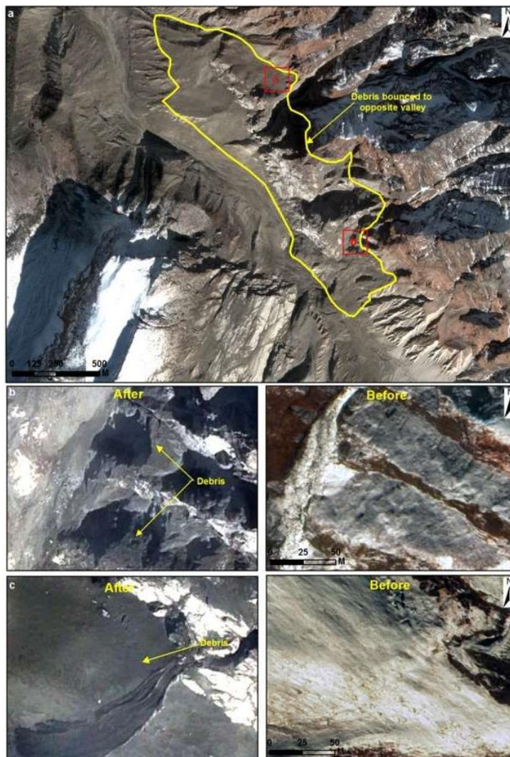
Figure 19: a. Zone of debris deposition on the opposite valley shown over the post-event Pleiades image. b. and c. show after and before images of debris deposition
