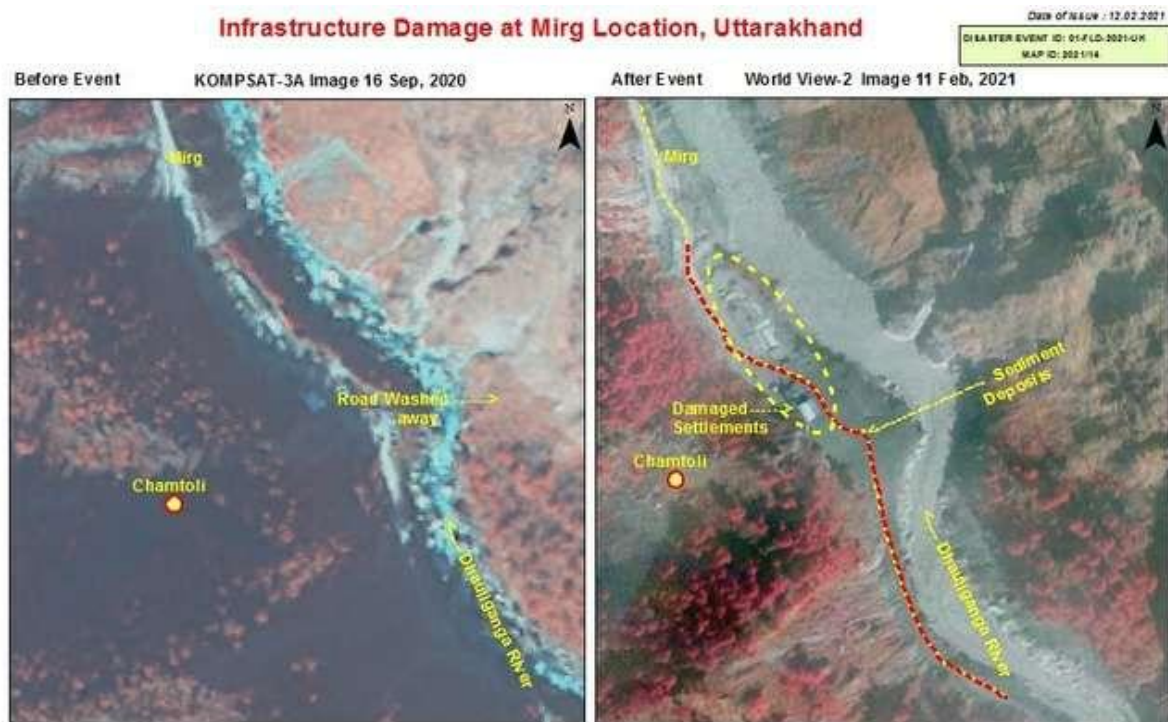
Figure 14: Damages to infrastructure in Mirg as on 11 th February 2021 (Source: NRSC-ISRO)
